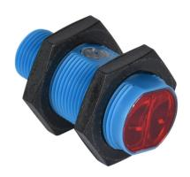
Contrinex photoelectric sensor, tubular, threaded, diffuse, visible red, 3-1200mm sensing distance, complementary light-on/dark-on, NPN, potentiometer, 1.5 kHz switching frequency, ABS plastic housing, 4-pin M12 quick-disconnect.
