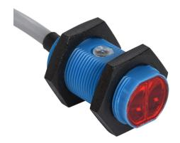
Contrinex photoelectric sensor, tubular, threaded, diffuse, visible red, 3-1200mm sensing distance, complementary light-on/dark-on, PNP, potentiometer, 1.5 kHz switching frequency, ABS plastic housing, pigtail.
