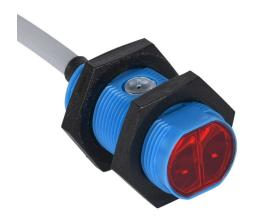
Contrinex photoelectric sensor, tubular, threaded, diffuse, visible red light emission, 3-1200mm sensing distance, complementary light-on/dark-on, NPN, potentiometer, 1.5 kHz switching frequency, ABS plastic housing, pigtail.
