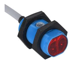
Contrinex photoelectric sensor, tubular, threaded, diffuse, visible red, 3-1200mm sensing distance, complementary light-on/dark-on, NPN, potentiometer, 1.5 kHz switching frequency, ABS plastic housing, pigtail.
