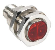
Contrinex photoelectric sensor, tubular, threaded, diffuse, visible red, 3-1200mm sensing distance, complementary light-on/darkon, PNP, potentiometer, 1.5 kHz switching frequency, stainless steel housing, 4-pin M12 quick-disconnect.
