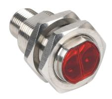
Contrinex photoelectric sensor, tubular, threaded, diffuse, visible red, 3-1200mm sensing distance, complementary light-on/dark-on, NPN, potentiometer, 1.5 kHz switching frequency, stainless steel housing, 4-pin M12 quick-disconnect.
