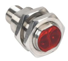
Contrinex photoelectric sensor, tubular, threaded, diffuse, visible red light emission, 3-1200mm sensing distance, complementary light-on/dark-on, NPN, potentiometer, 1.5 kHz switching frequency, stainless steel housing, 4-pin M12 quick-disconnect.
