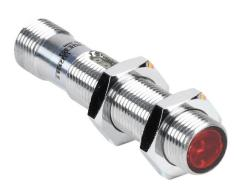
Contrinex photoelectric sensor, tubular, threaded, diffuse, visible red, 5-800mm sensing distance, complementary light-on/dark-on, PNP, potentiometer, 1.5 kHz switching frequency, chrome-plated brass housing, 4-pin M12 quick-disconnect.
