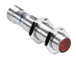
Contrinex photoelectric sensor, tubular, threaded, diffuse, visible red light emission, 5-800mm sensing distance, complementary light-on/dark-on, PNP, potentiometer, 1.5 kHz switching frequency, chrome-plated brass housing, 4-pin M12 quick-disconnect.
