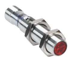
Contrinex photoelectric sensor, tubular, threaded, diffuse, visible red, 5-800mm sensing distance, complementary light-on/dark-on, NPN, potentiometer, 1.5 kHz switching frequency, chrome-plated brass housing, 4-pin M12 quick-disconnect.
