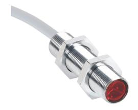
Contrinex photoelectric sensor, tubular, threaded, diffuse, visible red light emission, 5-800mm sensing distance, complementary light-on/dark-on, PNP, potentiometer, 1.5 kHz switching frequency, chrome-plated brass housing, pigtail.
