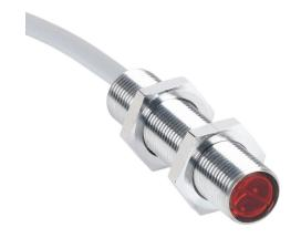
Contrinex photoelectric sensor, tubular, threaded, diffuse, visible red, 5-800mm sensing distance, complementary light-on/dark-on, PNP, potentiometer, 1.5 kHz switching frequency, chrome-plated brass housing, pigtail.
