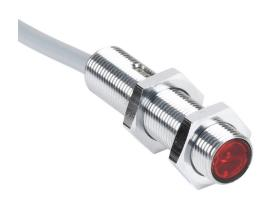
Contrinex photoelectric sensor, tubular, threaded, diffuse, visible red, 5-800mm sensing distance, complementary light-on/dark-on, NPN, potentiometer, 1.5 kHz switching frequency, chrome-plated brass housing, pigtail.
