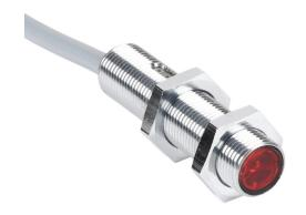
Contrinex photoelectric sensor, tubular, threaded, diffuse, visible red light emission, 5-800mm sensing distance, complementary light-on/dark-on, NPN, potentiometer, 1.5 kHz switching frequency, chrome-plated brass housing, pigtail.
