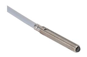
Contrinex photoelectric sensor, tubular, threaded, diffuse, visible red, 0-120mm sensing distance, light-on, PNP, teach-in wire, 1 kHz switching frequency, stainless steel housing, pigtail.
