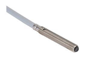
Contrinex photoelectric sensor, tubular, threaded, diffuse, visible red light emission, 0-120mm sensing distance, light-on, PNP, teach-in wire, 1 kHz switching frequency, stainless steel housing, pigtail.
