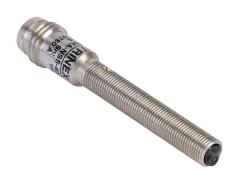
Contrinex photoelectric sensor, tubular, threaded, diffuse, visible red, 0-12mm sensing distance, light-on, PNP, 1 kHz switching frequency, stainless steel housing, 3-pin M8 quick-disconnect.
