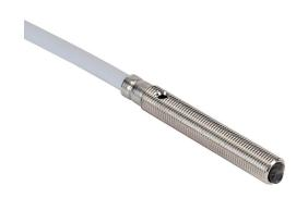
Contrinex photoelectric sensor, tubular, threaded, diffuse, visible red light emission, 0-12mm sensing distance, light-on, PNP, 1 kHz switching frequency, stainless steel housing, pigtail.
