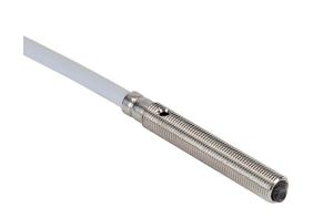
Contrinex photoelectric sensor, tubular, threaded, diffuse, visible red, 0-12mm sensing distance, light-on, PNP, 1 kHz switching frequency, stainless steel housing, pigtail.
