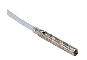
Contrinex photoelectric sensor, tubular, threaded, diffuse, visible red, 0-12mm sensing distance, light-on, NPN, 1 kHz switching frequency, stainless steel housing, pigtail.
