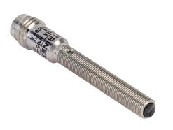
Contrinex photoelectric sensor, tubular, threaded, diffuse, visible red, 0-24mm sensing distance, light-on, PNP, 1 kHz switching frequency, stainless steel housing, 3-pin M8 quick-disconnect.
