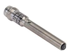
Contrinex photoelectric sensor, tubular, threaded, diffuse, visible red, 0-24mm sensing distance, light-on, NPN, 1 kHz switching frequency, stainless steel housing, 3-pin M8 quick-disconnect.
