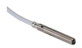
Contrinex photoelectric sensor, tubular, threaded, diffuse, visible red, 0-24mm sensing distance, light-on, PNP, 1 kHz switching frequency, stainless steel housing, pigtail.
