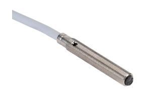
Contrinex photoelectric sensor, tubular, threaded, diffuse, visible red, 0-24mm sensing distance, light-on, NPN, 1 kHz switching frequency, stainless steel housing, pigtail.
