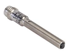
Contrinex photoelectric sensor, tubular, threaded, diffuse, visible red, 0-60mm sensing distance, light-on, PNP, 1 kHz switching frequency, stainless steel housing, 3-pin M8 quick-disconnect.
