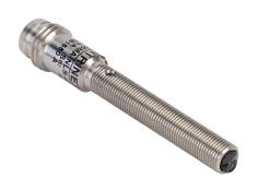
Contrinex photoelectric sensor, tubular, threaded, diffuse, visible red light emission, 0-60mm sensing distance, light-on, PNP, 1 kHz switching frequency, stainless steel housing, 3-pin M8 quick-disconnect.
