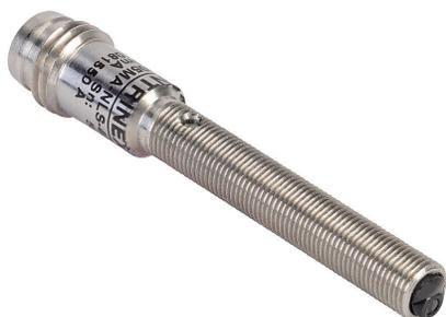
Contrinex photoelectric sensor, tubular, threaded, diffuse, visible red, 0-60mm sensing distance, light-on, PNP, 1 kHz switching frequency, stainless steel housing, 3-pin M8 quick-disconnect.
