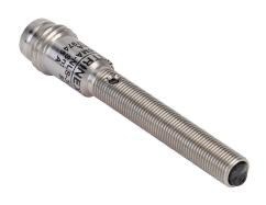
Contrinex photoelectric sensor, tubular, threaded, diffuse, visible red light emission, 0-60mm sensing distance, light-on, NPN, 1 kHz switching frequency, stainless steel housing, 3-pin M8 quick-disconnect.
