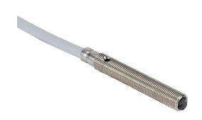
Contrinex photoelectric sensor, tubular, threaded, diffuse, visible red, 0-60mm sensing distance, light-on, PNP, 1 kHz switching frequency, stainless steel housing, pigtail.
