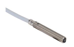
Contrinex photoelectric sensor, tubular, threaded, diffuse, visible red, 0-60mm sensing distance, light-on, NPN, 1 kHz switching frequency, stainless steel housing, pigtail.
