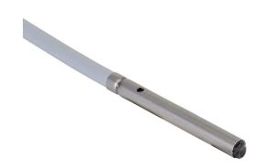
Contrinex photoelectric sensor, tubular, smooth, diffuse, visible red, 0-120mm sensing distance, light-on, PNP, teach-in wire, 1 kHz switching frequency, stainless steel housing, pigtail.
