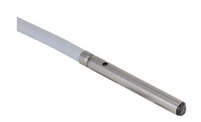
Contrinex photoelectric sensor, tubular, smooth, diffuse, visible red, 0-120mm sensing distance, light-on, NPN, teach-in wire, 1 kHz switching frequency, stainless steel housing, pigtail.
