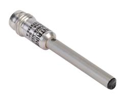
Contrinex photoelectric sensor, tubular, smooth, diffuse, visible red, 0-12mm sensing distance, light-on, PNP, 1 kHz switching frequency, stainless steel housing, 3-pin M8 quick-disconnect.
