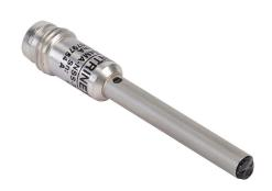
Contrinex photoelectric sensor, tubular, smooth, diffuse, visible red, 0-12mm sensing distance, light-on, NPN, 1 kHz switching frequency, stainless steel housing, 3-pin M8 quick-disconnect.
