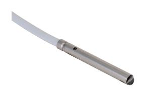
Contrinex photoelectric sensor, tubular, smooth, diffuse, visible red, 0-12mm sensing distance, light-on, PNP, 1 kHz switching frequency, stainless steel housing, pigtail.
