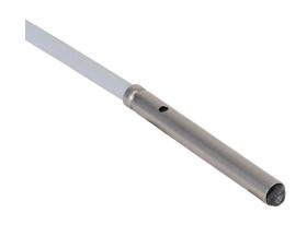
Contrinex photoelectric sensor, tubular, smooth, diffuse, visible red, 0-12mm sensing distance, light-on, NPN, 1 kHz switching frequency, stainless steel housing, pigtail.
