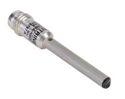
Contrinex photoelectric sensor, tubular, smooth, diffuse, visible red, 0-24mm sensing distance, light-on, PNP, 1 kHz switching frequency, stainless steel housing, 3-pin M8 quick-disconnect.
