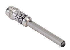
Contrinex photoelectric sensor, tubular, smooth, diffuse, visible red light emission, 0-24mm sensing distance, light-on, NPN, 1 kHz switching frequency, stainless steel housing, 3-pin M8 quick-disconnect.
