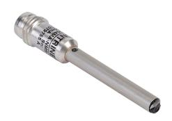
Contrinex photoelectric sensor, tubular, smooth, diffuse, visible red, 0-24mm sensing distance, light-on, NPN, 1 kHz switching frequency, stainless steel housing, 3-pin M8 quick-disconnect.
