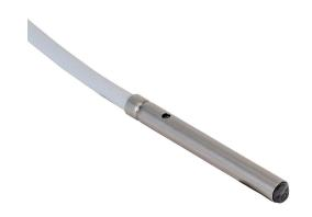
Contrinex photoelectric sensor, tubular, smooth, diffuse, visible red light emission, 0-24mm sensing distance, light-on, PNP, 1 kHz switching frequency, stainless steel housing, pigtail.
