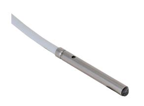
Contrinex photoelectric sensor, tubular, smooth, diffuse, visible red, 0-24mm sensing distance, light-on, PNP, 1 kHz switching frequency, stainless steel housing, pigtail.
