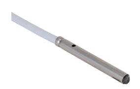
Contrinex photoelectric sensor, tubular, smooth, diffuse, visible red, 0-24mm sensing distance, light-on, NPN, 1 kHz switching frequency, stainless steel housing, pigtail.
