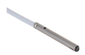
Contrinex photoelectric sensor, tubular, smooth, diffuse, visible red light emission, 0-24mm sensing distance, light-on, NPN, 1 kHz switching frequency, stainless steel housing, pigtail.
