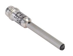
Contrinex photoelectric sensor, tubular, smooth, diffuse, visible red, 0-60mm sensing distance, light-on, PNP, 1 kHz switching frequency, stainless steel housing, 3-pin M8 quick-disconnect.
