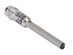
Contrinex photoelectric sensor, tubular, smooth, diffuse, visible red, 0-60mm sensing distance, light-on, NPN, 1 kHz switching frequency, stainless steel housing, 3-pin M8 quick-disconnect.
