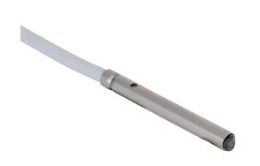
Contrinex photoelectric sensor, tubular, smooth, diffuse, visible red, 0-60mm sensing distance, light-on, PNP, 1 kHz switching frequency, stainless steel housing, pigtail.
