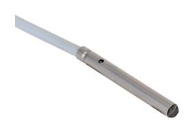
Contrinex photoelectric sensor, tubular, smooth, diffuse, visible red, 0-60mm sensing distance, light-on, NPN, 1 kHz switching frequency, stainless steel housing, pigtail.
