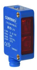
Contrinex photoelectric sensor, rectangular, diffuse, visible red, 5-1200mm sensing distance, complementary light-on/dark-on, PNP, potentiometer, 1.5 kHz switching frequency, ABS plastic housing, 4-pin M8 quick-disconnect.
