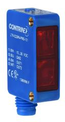
Contrinex photoelectric sensor, rectangular, diffuse, visible red light emission, 5-1200mm sensing distance, complementary light-on/dark-on, NPN, potentiometer, 1.5 kHz switching frequency, ABS plastic housing, 4-pin M8 quick-disconnect.
