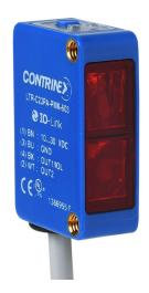
Contrinex photoelectric sensor, rectangular, diffuse, visible red, 5-1200mm sensing distance, complementary light-on/dark-on, PNP, potentiometer, 1.5 kHz switching frequency, ABS plastic housing, pigtail.
