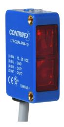
Contrinex photoelectric sensor, rectangular, diffuse, visible red, 5-1200mm sensing distance, complementary light-on/dark-on, NPN, potentiometer, 1.5 kHz switching frequency, ABS plastic housing, pigtail.
