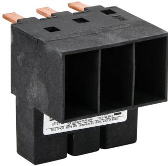
WEG Electric incoming power terminal block, 3-pole, maximum current 120A, 8-4 AWG. For use with MPW80 series manual motor protectors.
