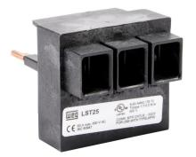
WEG Electric incoming power terminal block, 3-pole, maximum current 63A, 20-8 AWG. For use with MPW40 series manual motor protectors. Required when using a MPW40 in a UL Type E application 32A and less.
