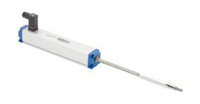
ProSense potentiometer linear position sensor, spring loaded slide, 100mm stroke,  $33 \times 33 \times 197$ mm body, channel mount, 8mm DIN 43650 Form C.
