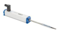
ProSense potentiometer linear position sensor, spring loaded slide, 75mm stroke, 33 x 33 x 172mm body, channel mount, 8mm DIN 43650 Form C.
