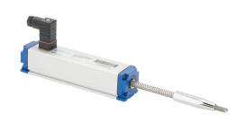
ProSense potentiometer linear position sensor, spring loaded slide, 50mm stroke, 33 x 33 x 147mm body, channel mount, 8mm DIN 43650 Form C.
