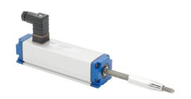
ProSense potentiometer linear position sensor, spring loaded slide, 30mm stroke, 33 x 33 x 127mm body, channel mount, 8mm DIN 43650 Form C.
