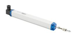
ProSense potentiometer linear position sensor, fixed slide, 200mm stroke,  $33 \times 33 \times 280$ mm body, channel mount, 18mm DIN 43650 Form A.
