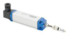
ProSense potentiometer linear position sensor, fixed slide, 50mm stroke, 33 x 33 x 130mm body, channel mount, 18mm DIN 43650 Form A.
