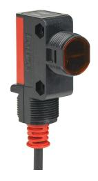
Leuze photoelectric sensor, rectangular, ABS plastic housing, through-beam emitter, infrared light emission, 0-10m sensing distance, 10-30 VDC operating voltage, 2-wire, pigtail.
