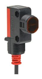
Leuze photoelectric sensor, rectangular, ABS plastic housing, through-beam emitter, infrared, 0-10m sensing distance, 10-30 VDC operating voltage, 2-wire, pigtail.
