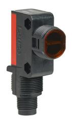
Leuze photoelectric sensor, rectangular, ABS plastic housing, through-beam emitter, visible red, 0-10m sensing distance, 10-30 VDC operating voltage, 2-wire, 4-pin M12 quick-disconnect.
