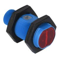
Contrinex photoelectric sensor, tubular, threaded, polarized retroreflective, visible red, 0.02-7m sensing distance, complementary light-on/dark-on, PNP, 4-wire, 4-pin M12 quick-disconnect.
