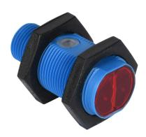
Contrinex photoelectric sensor, tubular, threaded, polarized retroreflective, visible red light emission, 0.02-7m sensing distance, complementary light-on/dark-on, PNP, 4-wire, 4-pin M12 quick-disconnect.
